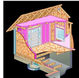
Using proven PINK FIBERGLAS™ blown-in insulation, combined with a PINK foam-based sealant, the EnergyComplete™ system delivers advanced energy efficiency and acoustical performance.
